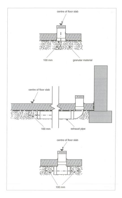
As part of the Soil Gas Control methods listed under Section 9.13.4 of the National Building Code, Rough-in for a subfloor depressurization system is required to allow for a future Radon extraction system if the need arises. Pipe is to be 100mm (4") ABS or PVC and installed within the gravel layer as shown in the detail.
